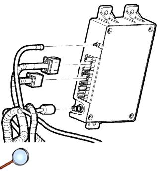
3. Disconnect the electrical connectors, the GPS antenna, and the cellular coax cable.
